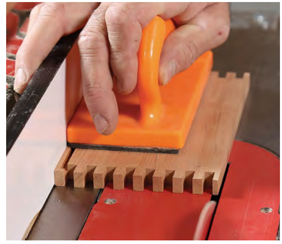
Trim the excess. Stowe cuts the fingers in stock that is a little wide and rips it to width later. This lets him clean up any cumulative error, like the thin finger on the right, that may have crept in.
