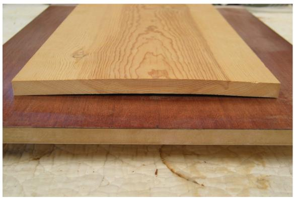
The first step is to turn the board over so it's bowed on the topside.
