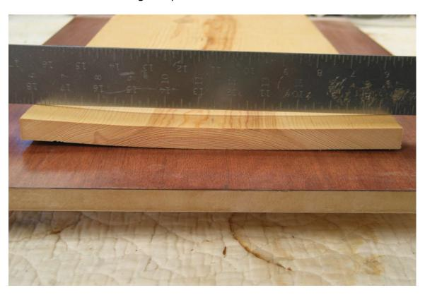
A typical pine board with inadequate kiln drying, so it shrunk and cupped on the outside of the rings as it dried more.
