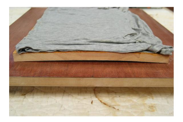
Then thoroughly wet this side with soaking wet cloths to make it swell.
