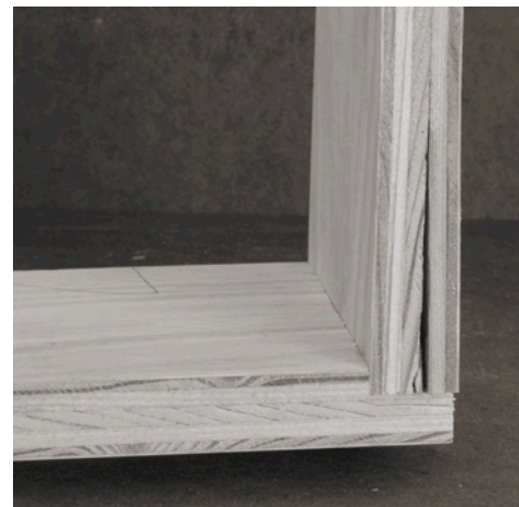
Fasteners driven in the edges of plywood can cause an inferior core to split, often delaminating adjacent layers.
