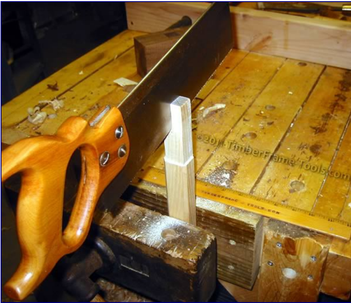
Sawing the wedge slot in the handle The final result should look like this.
