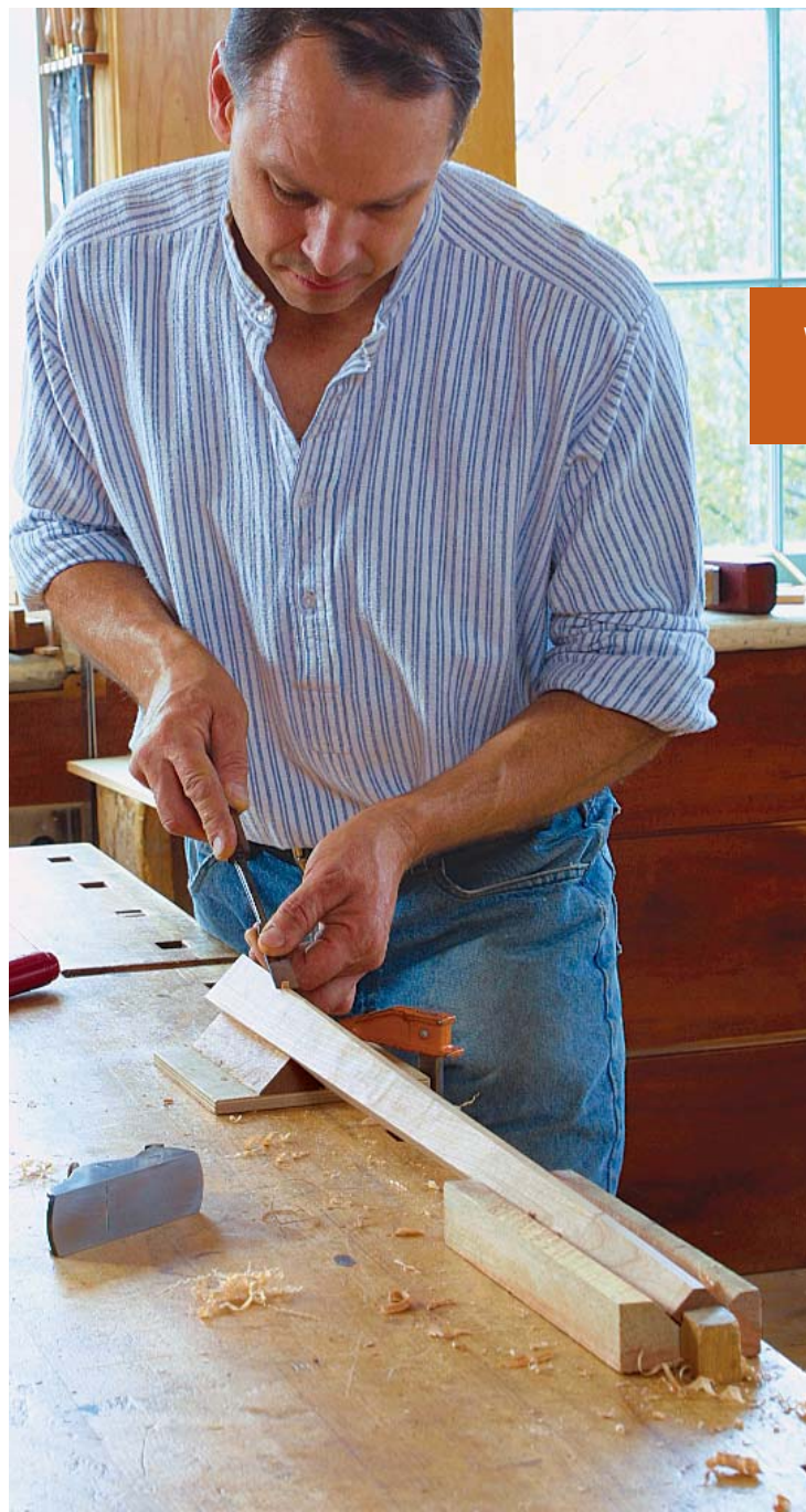
Planing thin, straight stock. This jig is simply a piece of plywood with thin, perpendicular fences. Butt the jig against a benchdog to hold it in place.
