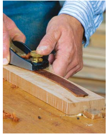
Planing thin, curved stock. A brass escutcheon pin tacked into a flat board serves as a ministop for smaller workpieces. Because brass is soft, it won't damage your tools if you run into it.
