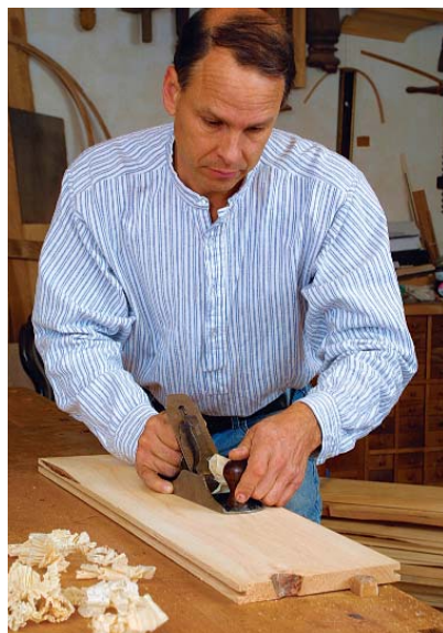
Planing against a single point. The easiest way to hold a board when planing is to use a single benchdog.
