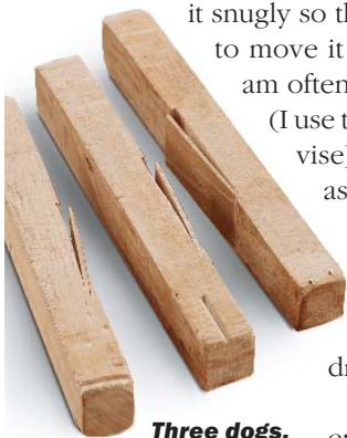
Three dogs. Adding pins or V-grooves to your dogs helps them hold thin or mitered stock.
