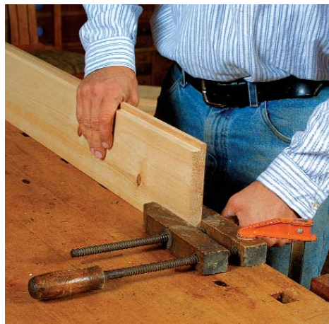
Wood hand screw holds long boards on edge. For longer, more unwieldy stock, use a hand screw clamped to the bench.
