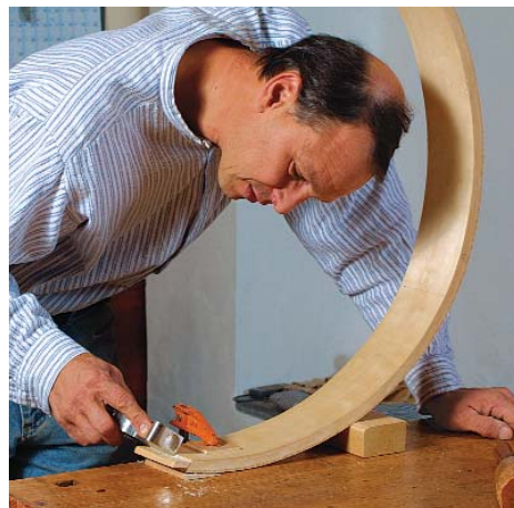
Tenon shaping on curved work. Use two wedges plus a clamp to keep the piece in place. If the larger block wants to move, place a benchdog behind it.
