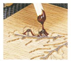
Tinted epoxy anchors the inlay into the recess. You only need a small amount to prevent squeezeout.
