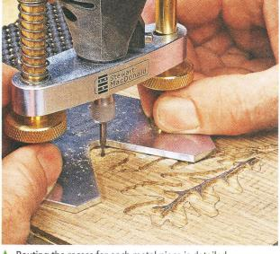
Routing the recess for each metal piece is detailed work. Using a small bit gives you the best control and allows you to work into tight corners.
