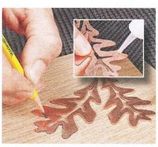
A couple of drops of thick instant glue will hold the inlay in place as you trace the pattern onto the workpiece.
