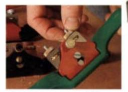
Tap or twist. All of the standard-angle shaves Gochnour tested allow for easy blade adjustments via thumbscrews on the lever cap (above) or with the tap of a hammer (below).
