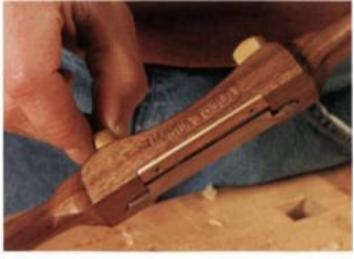
Two ways to adjust the blade. On some low-angle shaves, you have to remove the blade to change the depth of cut (far left). Other models (left) allow you to adjust the blade depth without removing the blade, a more convenient system.
