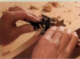
When pushing or pulling the shave, work with the grain. On a concave surface, that means starting at the ends and working downhill toward the middle. On a convex surface, work from the middle toward the ends.
