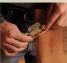
**Smooth cuts in rough areas.** Skewing the shave on end grain and tricky or reversing grain helps reduce the effective cutting angle of the tool, allowing for smooth cuts without chatter.
