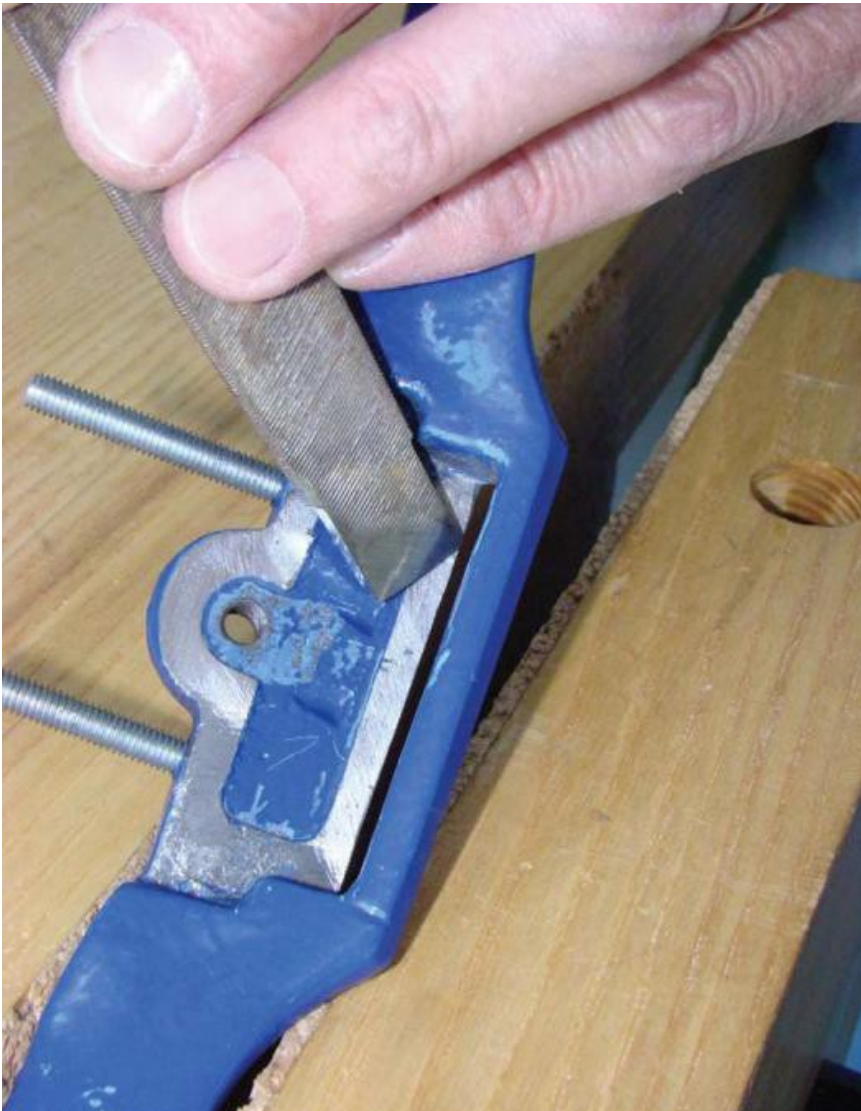
Painted Bed – The small dark spots to either side of the cap screw and around the mouth are the only points where the blade makes contact with the body. The paint needs to be removed and the bed scraped flat.
