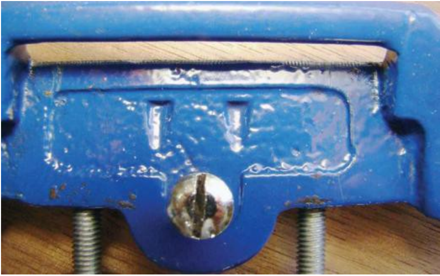
Painted Bed – The small dark spots to either side of the cap screw and around the mouth are the only points where the blade makes contact with the body. The paint needs to be removed and the bed scraped flat.
