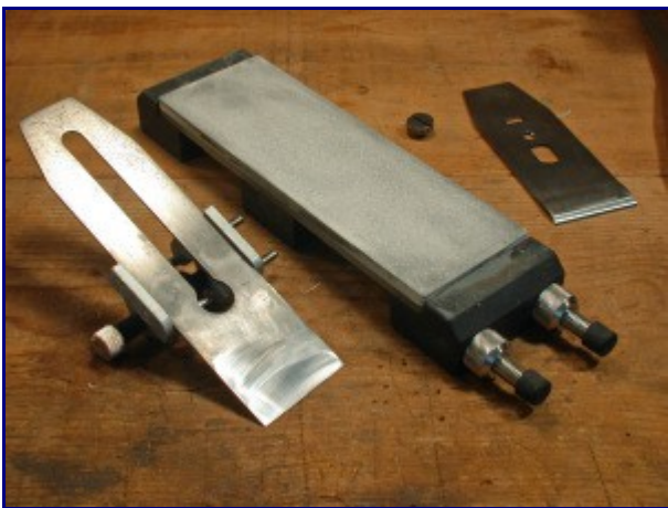
Basic sharpening setup using a waterstone
